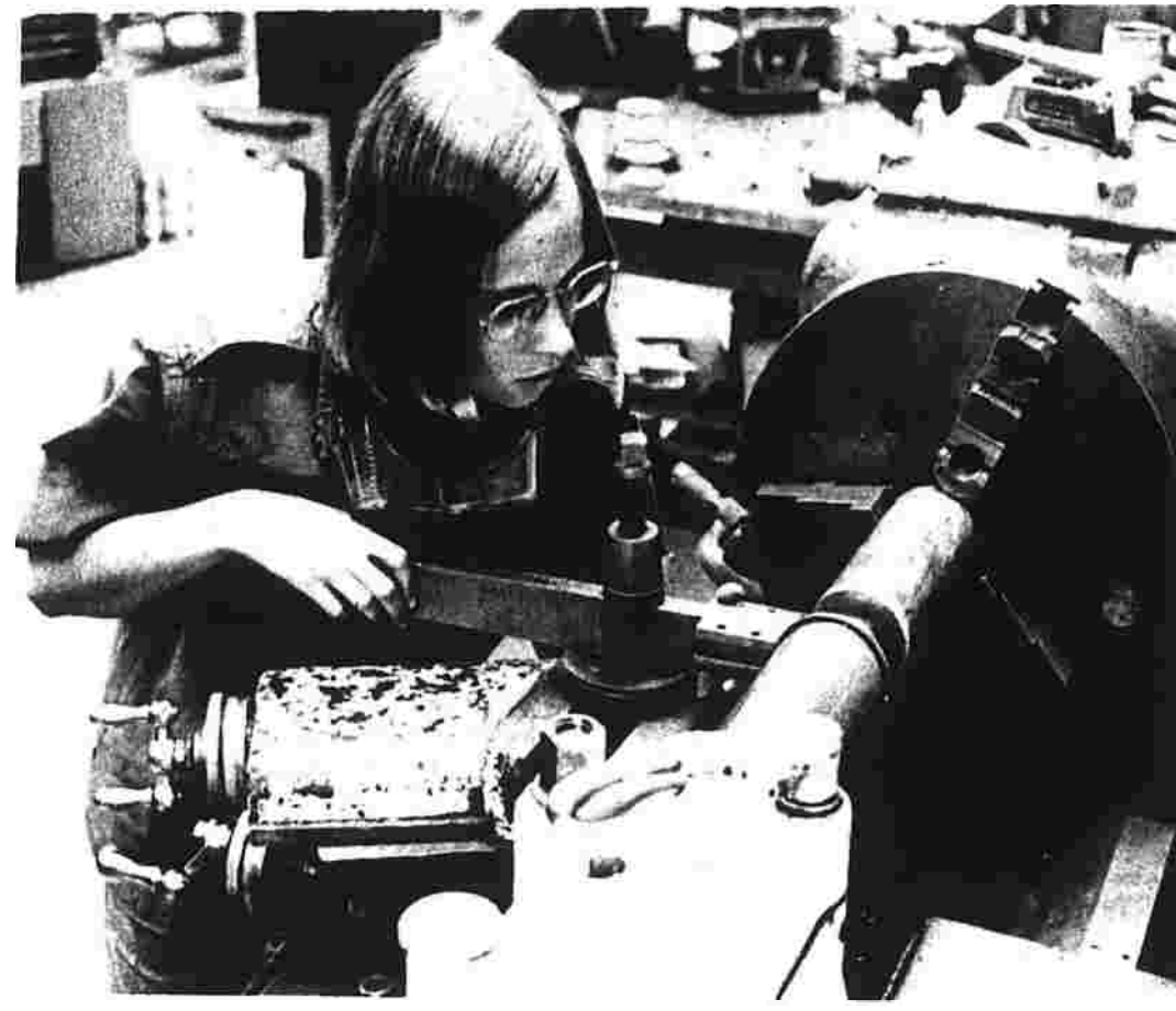
Pvt. 2 Laura Smith sizes up and makes adjustments in preparing this lathe to "turn down" a piece of metal. She indicated that this particular metal would later be made into a bushing remover. (U.S. Army Photo)
